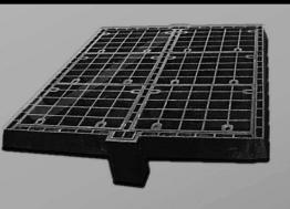
APEX Undergrounds range of Multi-part Access Covers are designed for use where manhole clear openings exceed 1200mm dimension. Multi-part covers incorporate removable support beams enabling large openings to be covered. Covers are sent flat pack for simple and cost effective transport.
