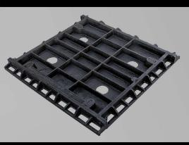
APEX Undergrounds range of Single Part Recessed Access Covers are manufactured from highly durable ductile iron, complete with fully machined mating surfaces between cover & frame. Designed with a unique polyethylene gasket within the frame assembly, our covers have eliminated the requirement for lead contaminated frame joints, while maintaining a gas and watertight seal.
