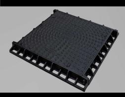
APEX Undergrounds range of Single Part Solid-top Access Covers are manufactured from highly durable ductile iron, complete with fully machined mating surfaces between cover & frame. Utilizing the antislip chevron pattern, the covers are safe, aesthetically pleasing and robust. Solid-top access covers are lighter in weight than traditional concrete infill and therefore are ideal where regular access is required.
